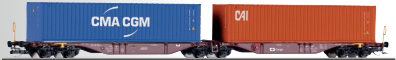
Containertragwagen Sggmrss 578.0 der ČD Cargo Container car Sggmrss 578.0 of the ČD Cargo
