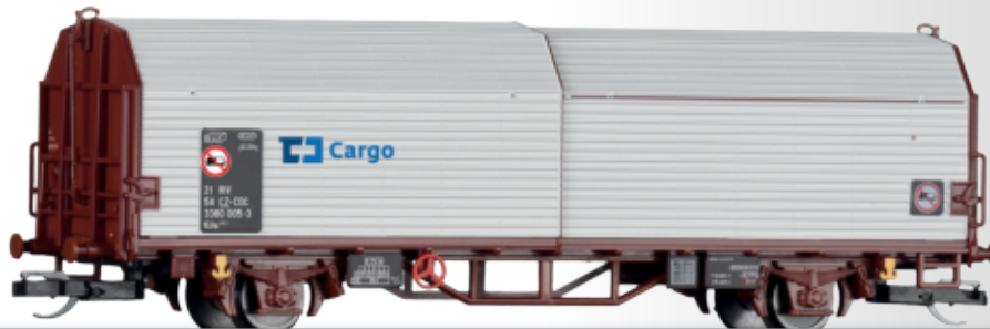
Haubenwagen Kils der ČD Cargo Hood car Kils of the ČD Cargo
