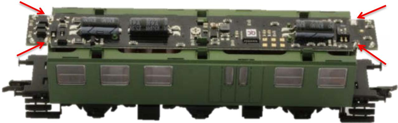
Solder the track connection to the circuit board
