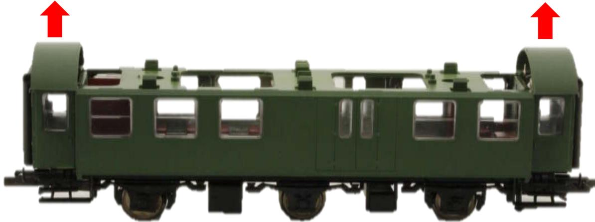
Pull the entry housing of the car in upper direction, as indicated by the arrows and remove the entry housing from the top of the body.
