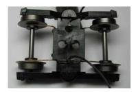
6. Guide the wire through longitudinal recess into the wagon's interior. Mount the bogies.
