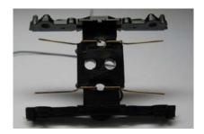
5. Install the wheel sets, align the contacts and solder on the wires:
