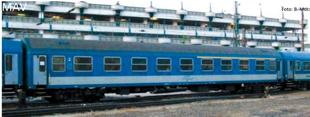
74759 III/2009 Reisezugwagen 1./2. Kl., Typ Y der MAV-START, 1st/2nd class coach type Y of the MAV-START
