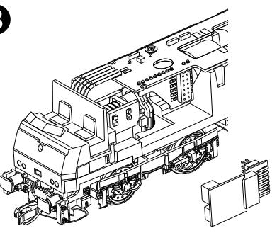
If the PluX12 decoder is used while in digital mode, it is possible to turn on the full beam autonomously. Also the locomotive rear light can be turned off individually or turned on without the front light is turned on. An additional rectangular loudspeaker can be installed in the area of the transformer replica. The loudspeaker is connected to the two soldering pads marked LSA and LSB on the main circuit board.
